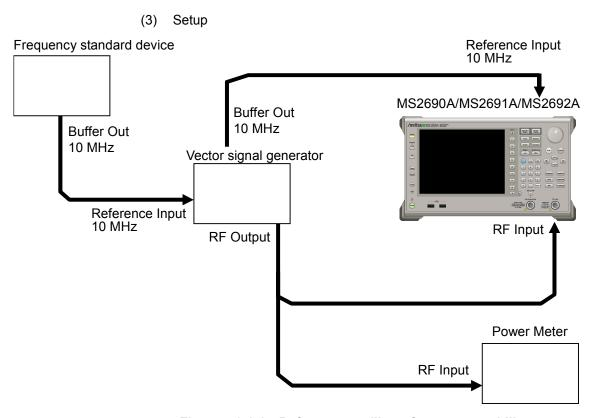
Figure 4.2.1-1 Reference oscillator frequency stability test
