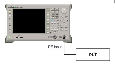
Figure 2.2-1 Signal path setup example
