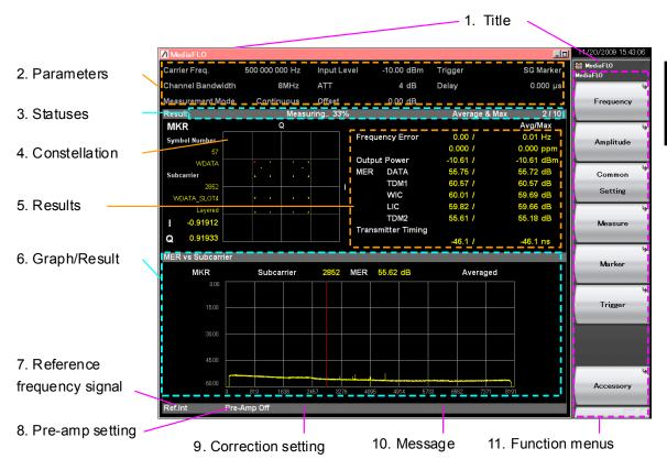
Figure 3.1.1-1 Screen Appearance (Modulation Analysis)
