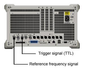
Figure 2.2-2 External signal input
